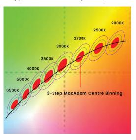
Nichia Chromaticity Diagram: Brownie Ecotronic is using the 3-Step MacAdam Centre Binning to ensure the excellent color consistency of our LED.
